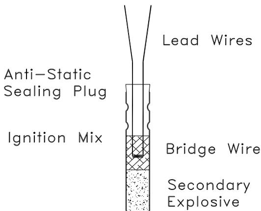
**Figure 1, Non-resistorized:**
