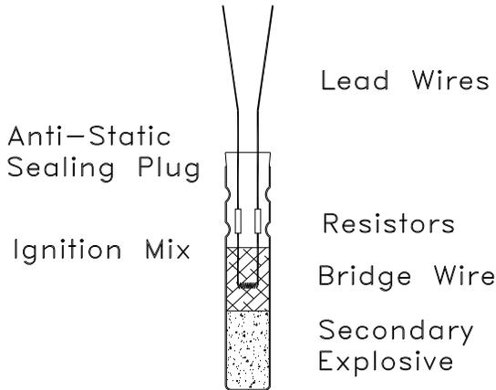
**Figure 2, Resistorized**
