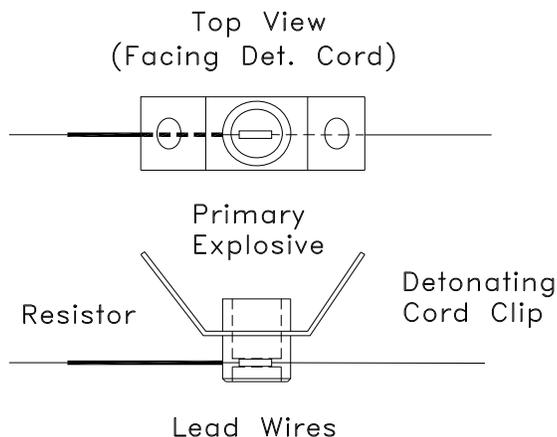
**Figure 4, Resistorized, Fluid Disabled**
